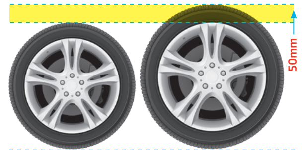
Diagram 2: Maximum wheel & tyre assembly diameter increase 50mm
